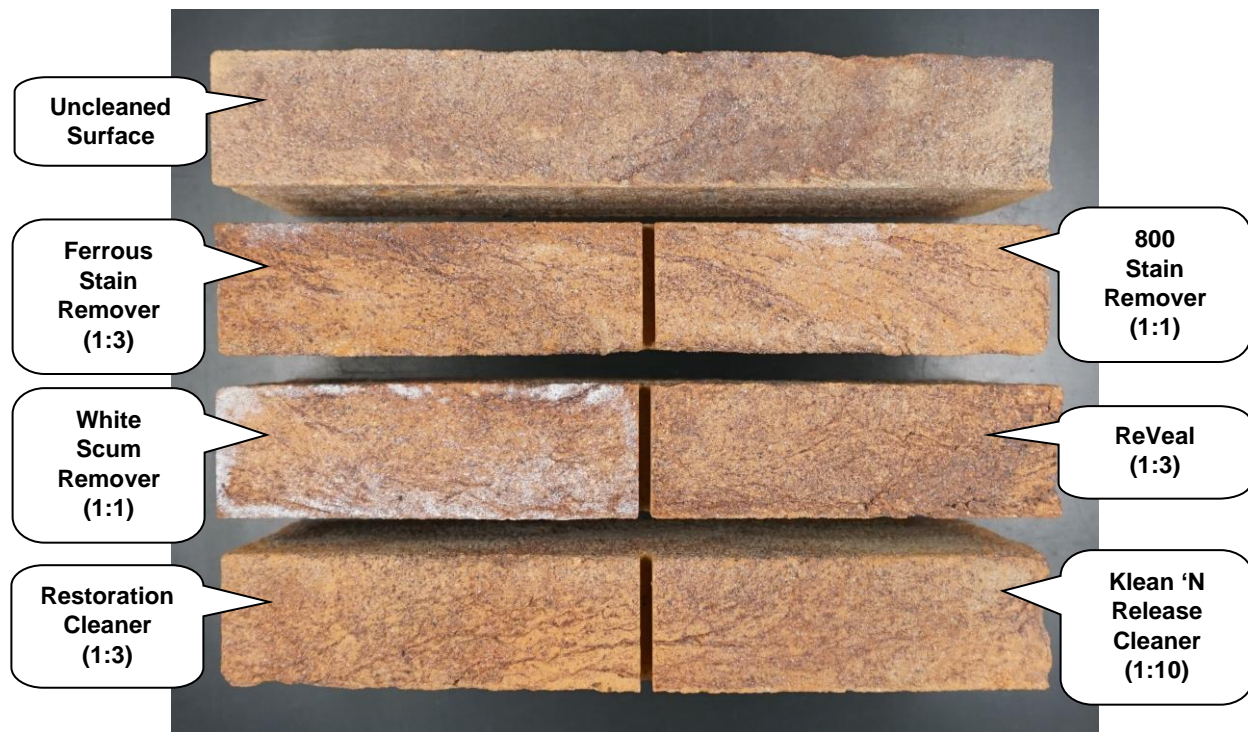
"Potenza Textured" Solid Brick After Cleaning
