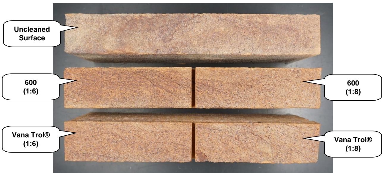
"Potenza Textured" Solid Brick After Cleaning
