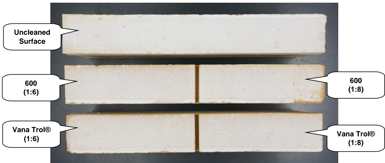
"Brenta Raw" Solid Brick After Cleaning
