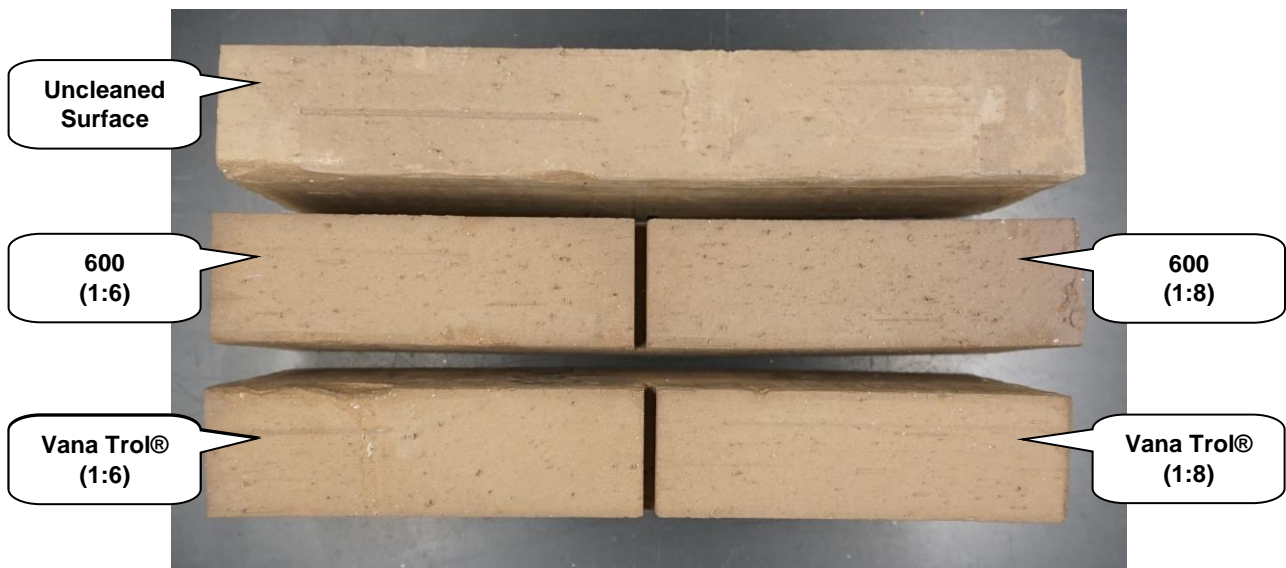
"Arno Raw" Solid Brick After Cleaning
