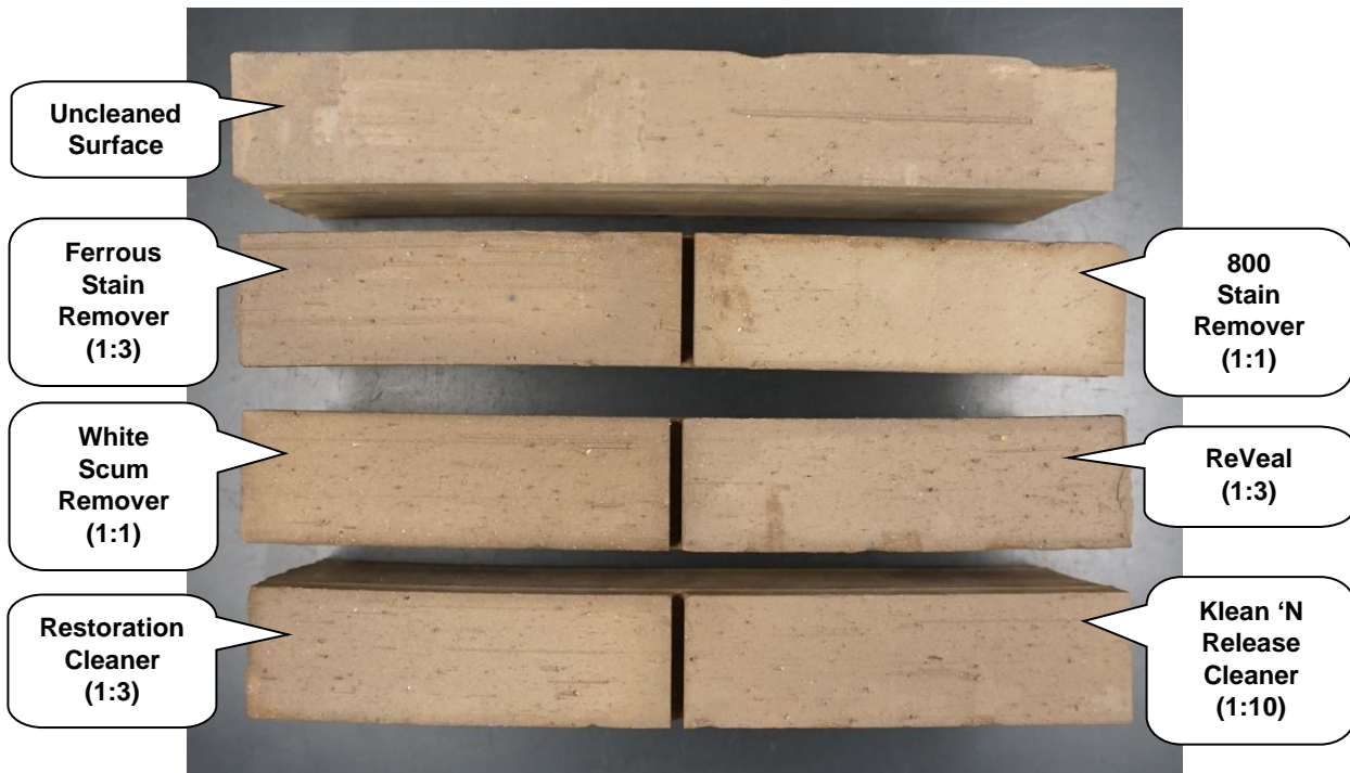
"Arno Raw" Solid Brick After Cleaning
