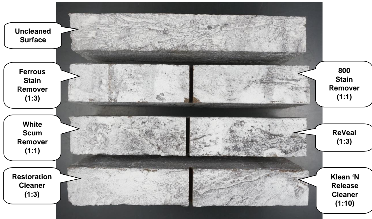
"Marana Textured" Solid Brick After Cleaning
