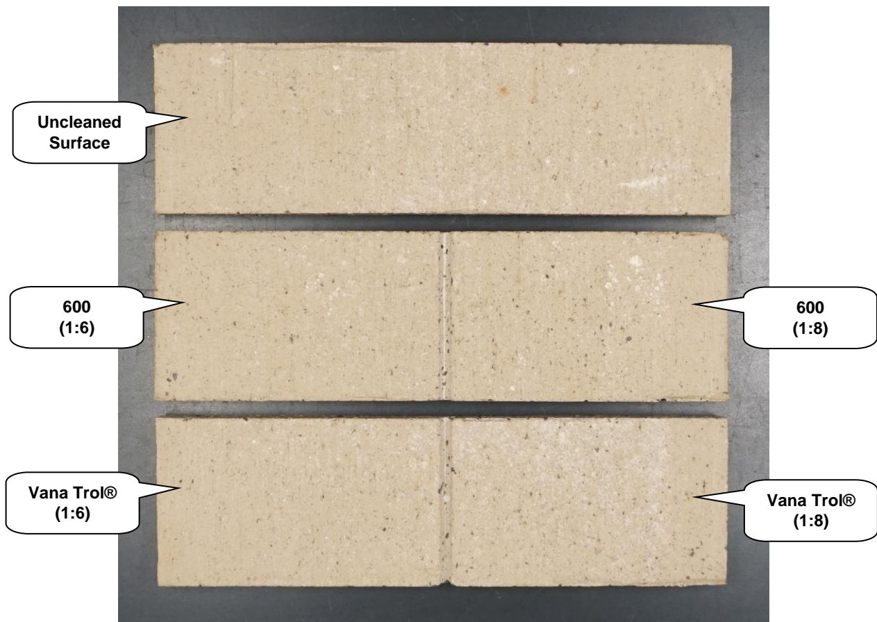
"Feldhaus 764 Gray White Waterstruck" Thin Brick After Cleaning
