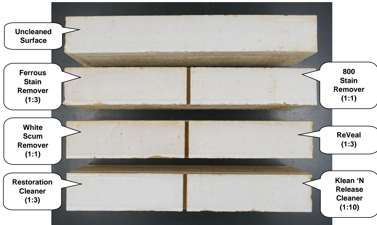
"Brenta Raw" Solid Brick After Cleaning
